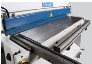
Full CE conformity protection with multi-beam light barriers and enclosures
